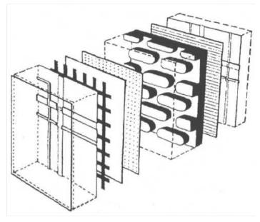
Image 5. Polyvalent wall by Mike Davis. The layers between the two glass panes are a thickness of a few microns.
